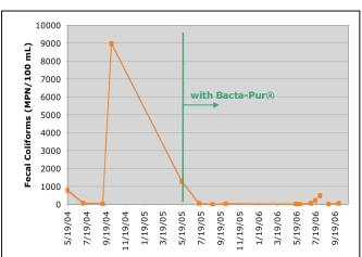
**Figure** 2. Fecal coliforms in the effluent. Use of Bacta-Pur®, helps keeping fecal coliforms below limit of 200 MPN/100 ml during the summer.
