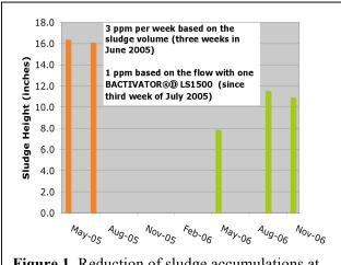
Figure 1. Reduction of sludge accumulations at the entrance of the first aerated lagoon.
